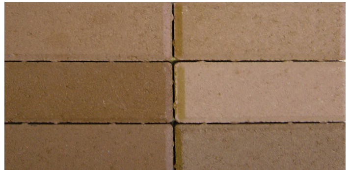
FIG.2: All pavers pigmented with PJ 4960 at 3%.
